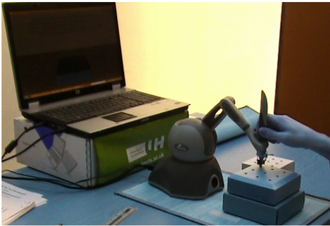
Fig. 3. This image shows the setup of the embedded reality version of the Nine Hole Peg Test. Attached to the end of the stylus is a peg, that allows the subject to experience real physical interactions, enhanced by haptic interactions that occur when the virtual stylus encounters the pegs and pegboard in the virtual environment.
